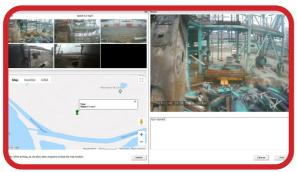
The SD cad can be removed from the vehicle so that the video footage can be reviewed on our bespoke analysis software which is designed to help the user quickly identify footage of interest, even when an accurate time and date is not known.
