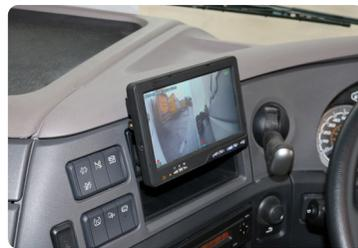
The LDVS systems include: Monitor, Nearside Side Camera, Nearside Proximity Detection System, Left Turn Alarm and Speed Turn On-Off Control Module. The FORS and CLOCS compliant systems adding a Reversing Camera to this system specification. All our Blind Spot Vision systems can be upgraded to the FORS GOLD Recording System specification as shown on the inside of this brochure.
