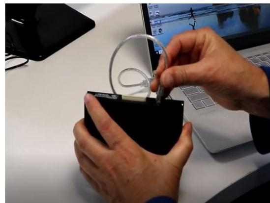
A drive can be removed and replaced with a spare drive, and the vehicle back in service, within 30 seconds.
