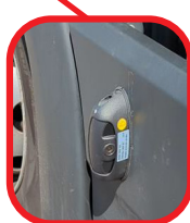
Vulnerable Road User Detection Camera
