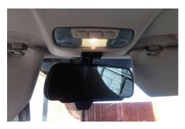
These DVR's can also be connected directly into a vehicle's infotainment system with adaptor leads available for many popular vehicles.
