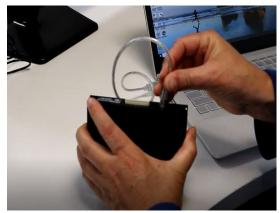
A drive can be removed and replaced with a spare drive, and the vehicle back in service, within 30 seconds.
