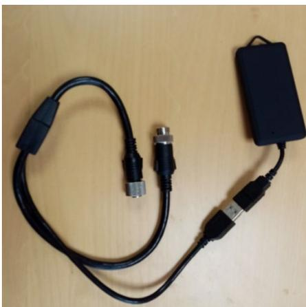
To calibrate and configure the VRUD Camera a Wi-Fi dongle has to be inserted in-line with the camera.
