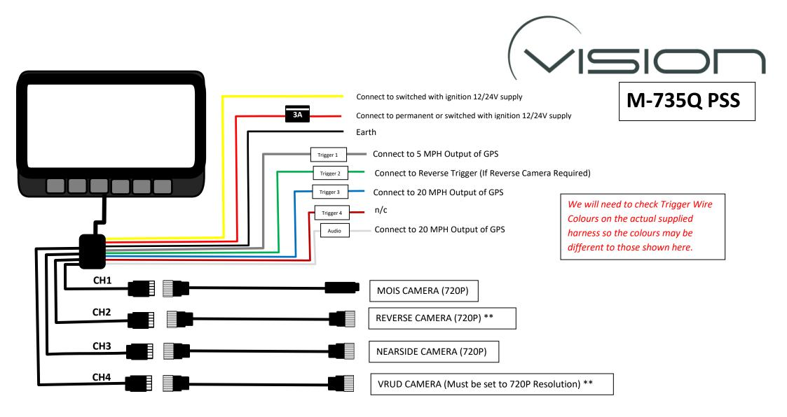
\*\* Cameras can be connected to any of the inputs and which cameras are displayed controlled by the trigger wires. For example, with the default configuration (shown above) - below 5MPH the Front Camera is shown on the Left of the Screen (CH1) and the Nearside Camera on the Right of the Screen (CH3). By connecting the Front Camera into CH3 and Left Camera into CH1, and Triggers connected accordingly, the Left Camera can be shown on the Left Side of the screen and the Front camera on the right.
